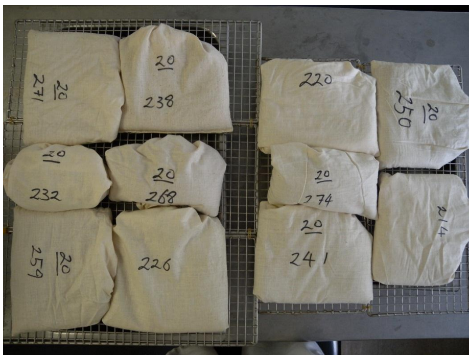
Figure 1 - Soybean meal samples packed in a calico bag and placed over sterilized water before entry to the Atherton Sterilizer.
