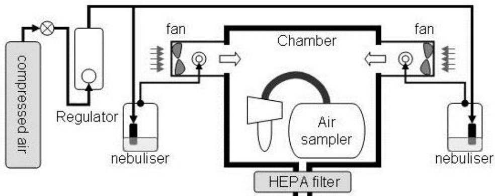
Figure 1: working diagram of a calibration chamber for air sampling.
