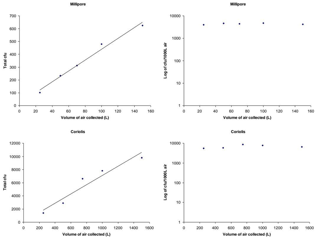
**Figure 5 - comparison of a plate impactor (top, Millipore) and a cyclonic air capture (bottom, Coriolis). Left: total number of cfu collected in a run. Right: bacterial concentrations per cubic meter of air (Logarithmic scale).**
