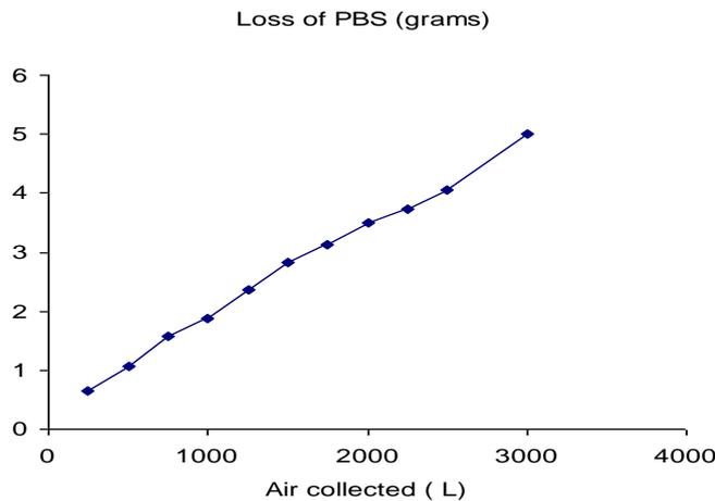
**Figure 2: loss of collecting buffer during air sampling.** The quantity of buffer present before and after sampling various volumes of air was determined by measuring the initial and final weights of the tubes. The weight difference is plotted against the total volume of air collected during each run.
